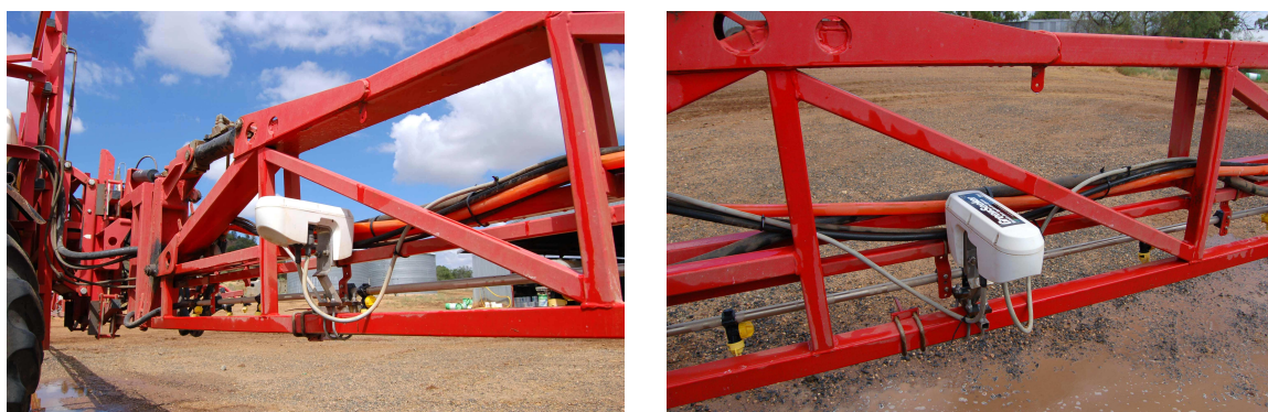
Photo 4.5.1: Photos of a Greenseeker RT200 sensor fitted to the spray rig boom (Photos courtesy of Richard Heath).
